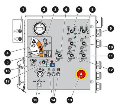
Status indicator pilot lights: These lights show the operation condition and errors in the control or engine functions.
