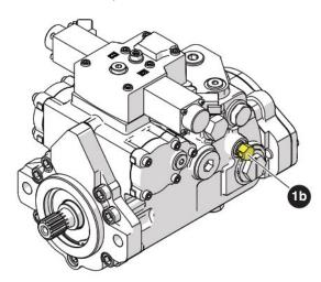
**1b Drive bypass valve with override stems** - This valve, when rotated counterclokwise by three full turns, is used to override the drive relief valves so the MEWP can be loaded or unloaded from a trailer with a winch line. Refer to *Section 6.4* for the winch and tow procedure.
