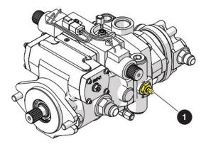
Orive bypass valve with override stems - This valve, when loosened 90 degrees clockwise, is used to override the drive relief valves so the MEWP can be loaded or unloaded from a trailer with a winch line. Refer to Section 6.4 for the winch and tow procedure.
