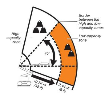
Figure 03 High and low-capacity zones
