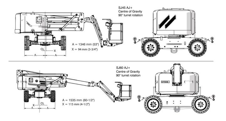
Figure 12 Lift points and center of gravity
