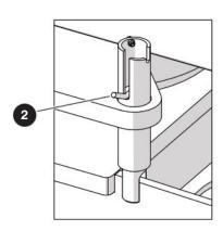
2 Turret transportation lock - This lock device is used to lock turret in position when you transport the MEWP. Refer to Section 6.6-1 for the procedure on how to lock the turret.
