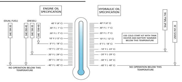
Figure 05 Cold weather operation chart
