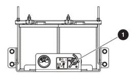
Main power disconnect: This switch disconnects power to all control circuits when it is in the off position. The switch must be in the on position to operate the MEWP. The switch must be in the off position when you transport the MEWP or put it in storage.
