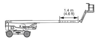
Figure 04 Fly boom extension into the low-capacity zone
