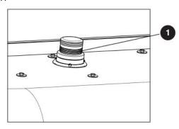
Flashing amber light: This light flashes when you operate a boom function. It operates with the motion alarm.
