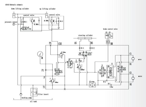
SS0407E Hydraulic schematic SS0507E Hydraulic schematic SS0607E Hydraulic schematic
