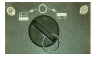
Fig. 22 Chassis control position
