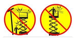
Maintain safe distances from electrical power lines and apparatus in accordance with
