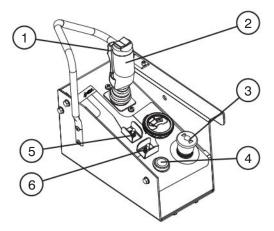
Figure 2-6. Platform Control Console with Toggle Switch
