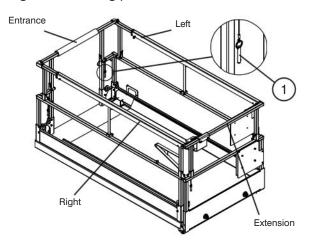
Figure 3-6. Folding Guardrail System
