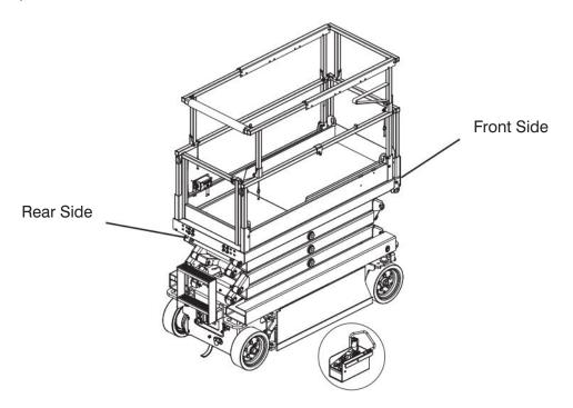
Figure 3-11. Control Box with Long Cable Outside Platform
