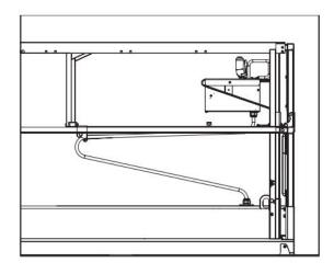
Figure 3-10. Control Box with Long Cable
