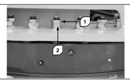
Check the turret fixing nuts on the slewing ring gear. Check for rusted, slackened or missing nuts. Contact your dealer in case of serious problems.
