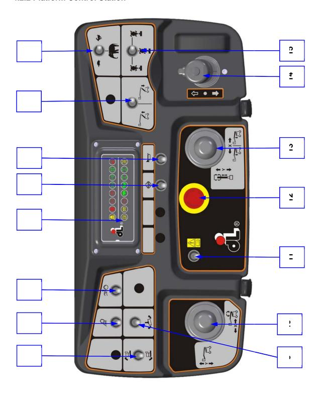
Figure 4-2 Platform Console Panel
