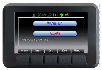
Figure 4-9 Alarm/Warning Interface
