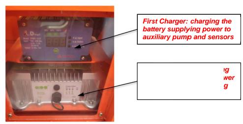
First charger, input voltage range: 100-240VAC, input current: 2.5A, frequency: 50-60Hz;
