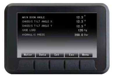
Figure 4-6 Vehicle Condition Interface
