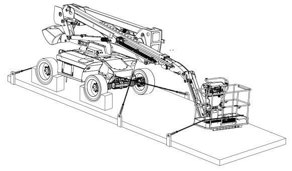
Figure 5-4 Tie Down Diagram
