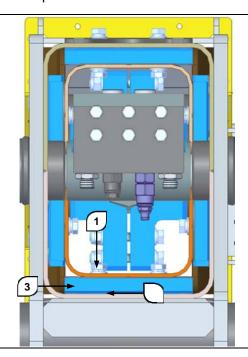
3) Slacken all the bolt 1 of the upper and lower sliding blocks of the first extension stage. If the space between the sliding surface of the block 3 and the sliding surface of the first boom exceeds 0.5mm, some pads 2 need to be added. And then tighten bolts 1.
