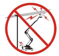
Maintain distance from electrical lines, apparatus, or any energized (exposed or insulated) parts according to the Minimum Approach Distance (MAD) as shown in Table 1.1
