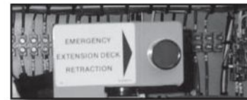
Figure 2-26. Emergency Powered Extension Platform Retraction System
