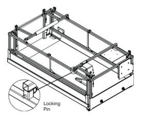
Figure 3-11c. All Guardrails Folded Down
