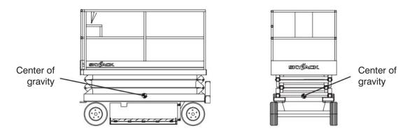
Figure 3-13. Center of Gravity
