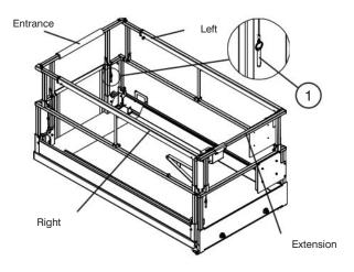
Figure 3-5. Folding Guardrail System
