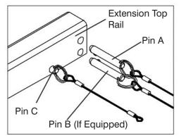
Figure 3-11b. Extension Top Rail Pins
