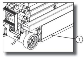
Figure 3-3. Pothole Protection Device
