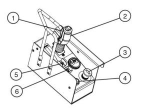
Figure 2-6. Platform Control Console
