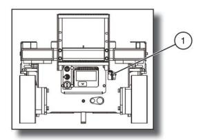
Figure 2-1. Main Power Disconnect Switch
