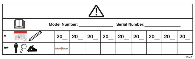
This decal is located on the scissor assembly. It must be completed after an annual inspection has been completed. Do not use the aerial platform if an inspection has not been recorded in the last 6 months.
