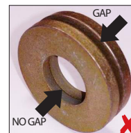
DO NOT FIT DISC SPRINGS LIKE THIS
