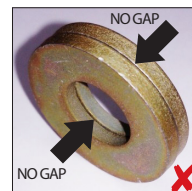
DO NOT FIT DISC SPRINGS LIKE THIS
