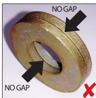
DO NOT FIT DISC SPRINGS LIKE THIS
