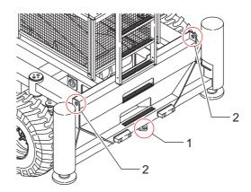
Towing, lashing and lifting eyes
