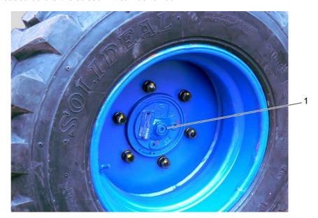
Bolt for the multiple disc brake
