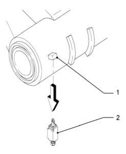
Lifting cylinder safety device
