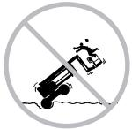
the machine in stowed position across uneven terrain, debris, unstable or slippery surfaces and near holes and drop-offs.
