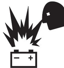
Keep sparks, flames and lighted tobacco away from batteries. Batteries emit explosive gas.
