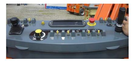
Photograph 2 - Platform control panel for another articulating boom
