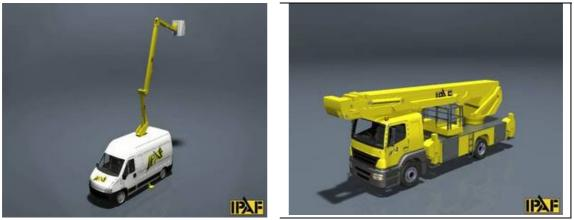
Photographs 6 & 7 Two different types of vehicle mounted boom (Source – www.ipaf.org)
