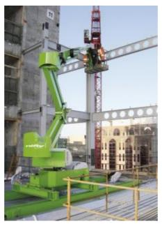
**Photograph 8** A deck mounted boom (Source – www.niftylift.com)
