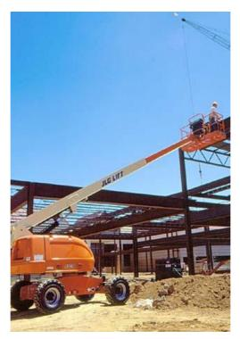
**Photograph 5** A telescopic boom (Source – www.jlg.com)
